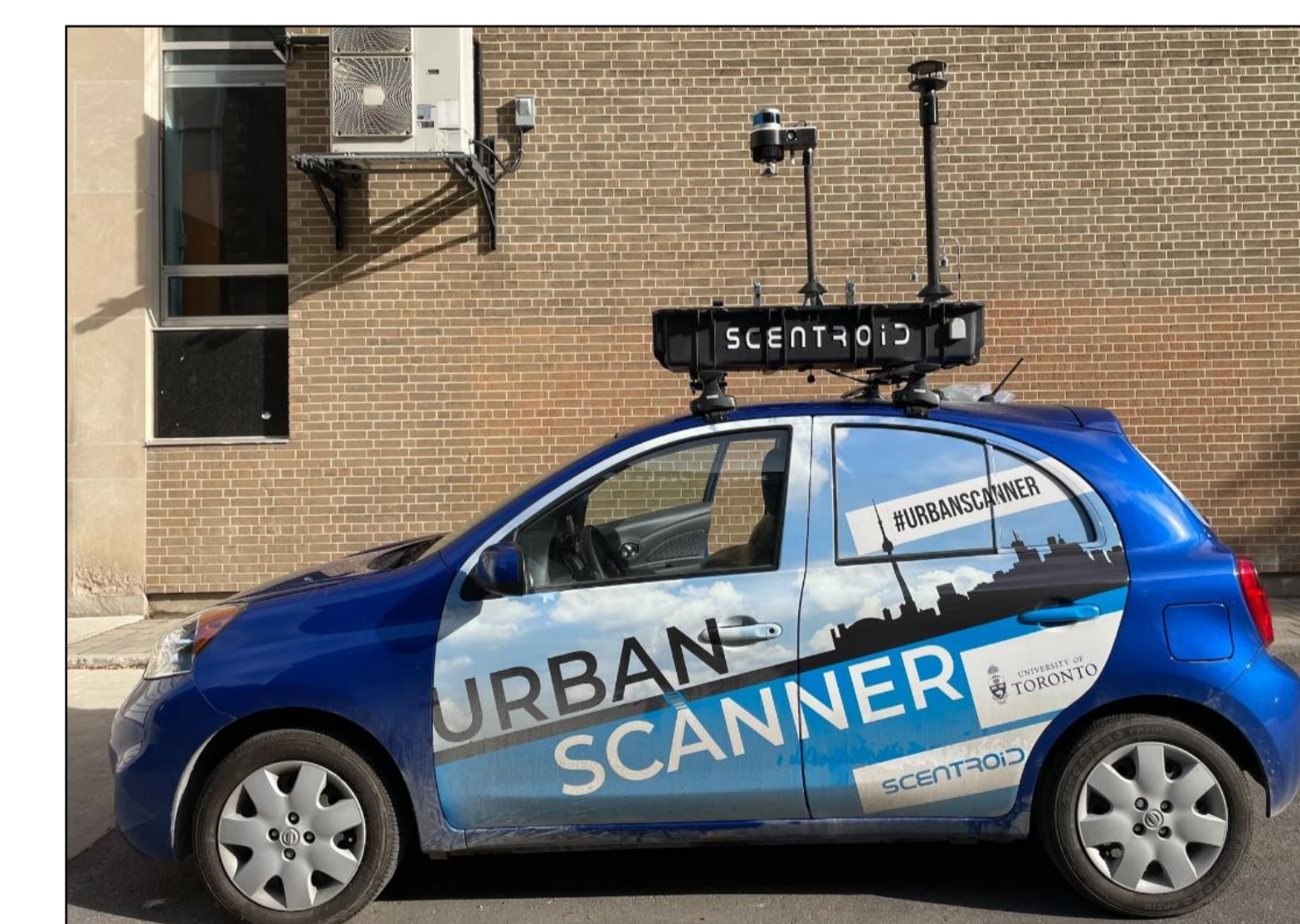
Figures: UrbanScanner mobile monitoring system. The vehicle is equipped with a computer, pollutant sensors, 360° camera, LiDAR, and meteorological probes.
